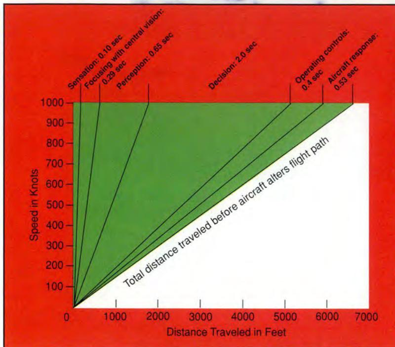
time to react to control inputs than smaller aircraft. For example, we'll use the F-15. This aircraft is capable of an instantaneous pitch rate of 22 degrees per second with maximum control deflection. Assuming a 0.5-second aircraft response to control inputs and a 5,000-foot turning radius at 450 knots, 0.52 seconds are required to move the aircraft 20 feet to avoid a bird strike. At 300 knots, 0.53 seconds are required for the same 20-foot movement in the airspace.
